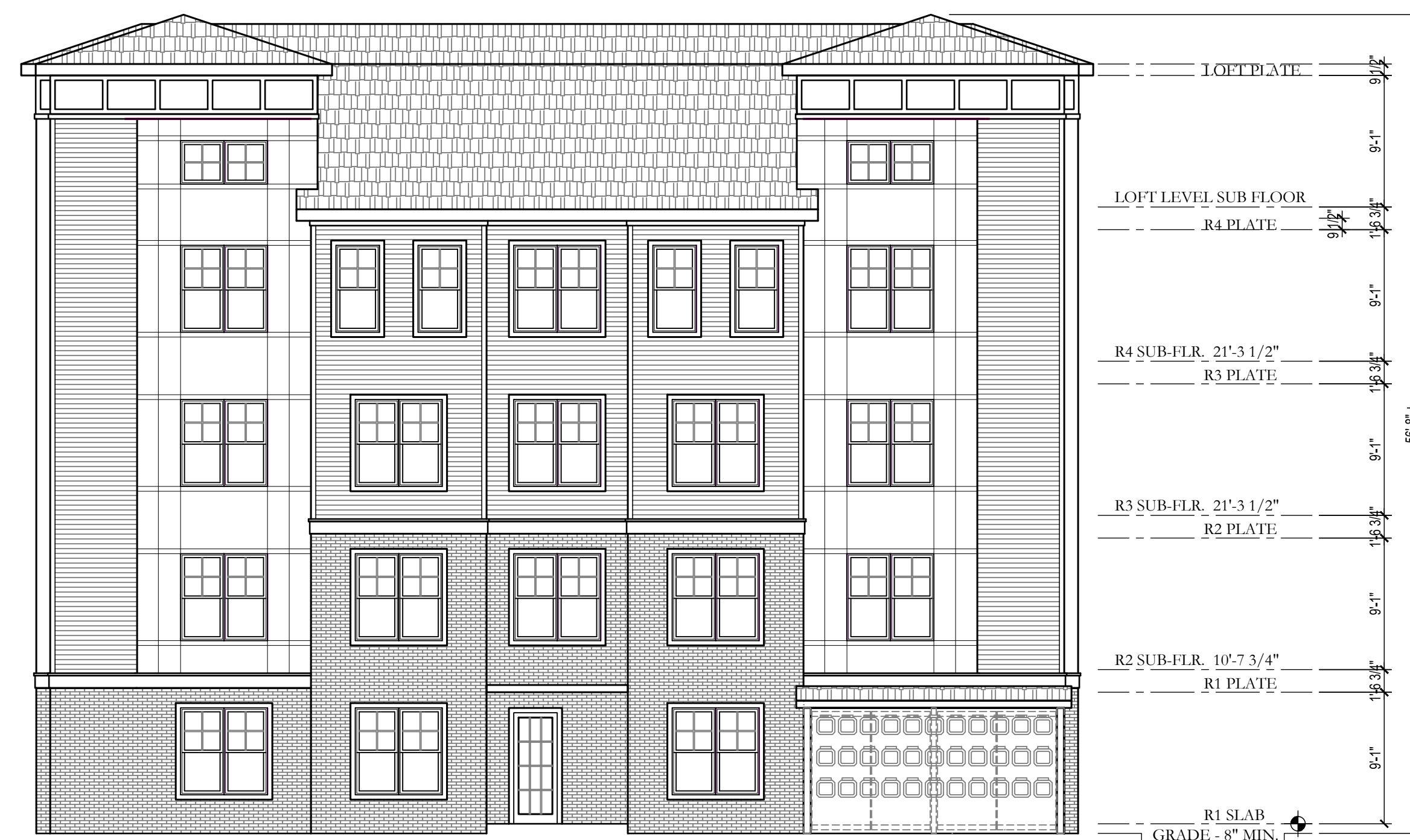
10 BUILDING 3 - RIGHT SIDE ELEVATION SCALE: 1/8" = 1'-0"
