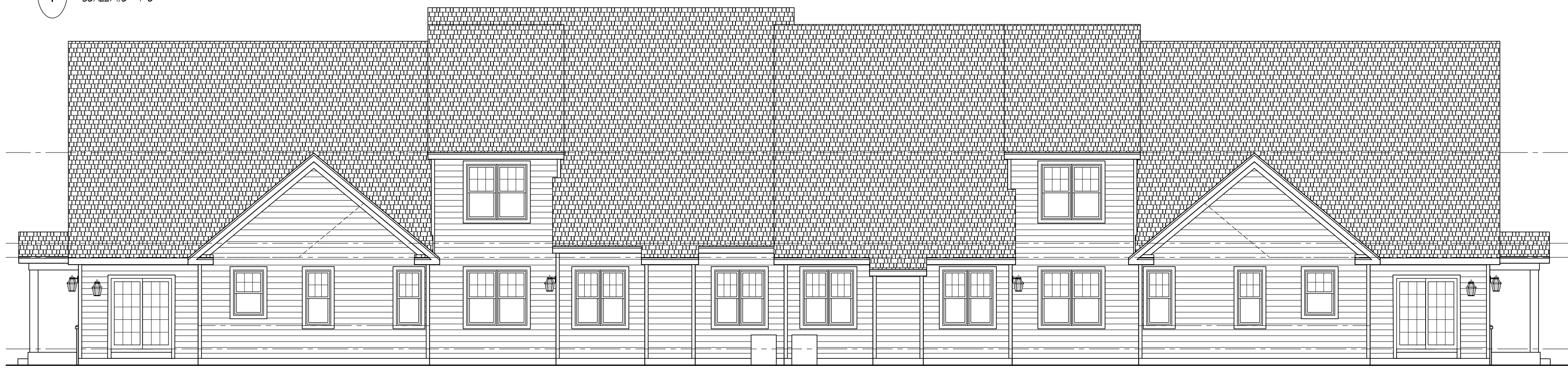
3 BUILDING TYPE D - REAR ELEVATION - STYLE 1 SCALE: 1/8" = 1'-0"
